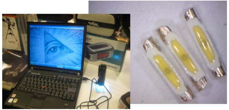
Left: handheld, USB powered microscope and camera, Right: picture of LEDs taken in court
